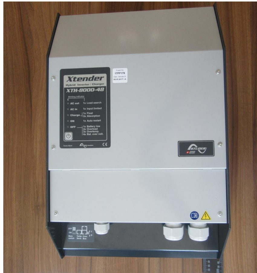
Front side enclosure of the unit (additional warning mark required, see next picture).
